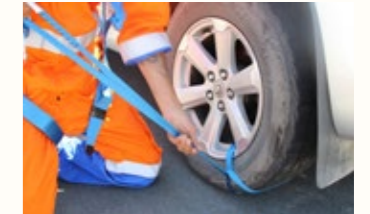
Anchor Point using Endless Sling:
