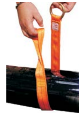
1. Place webbing sling around object.
