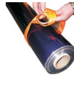
2. Feed metal ring through webbing loop.
