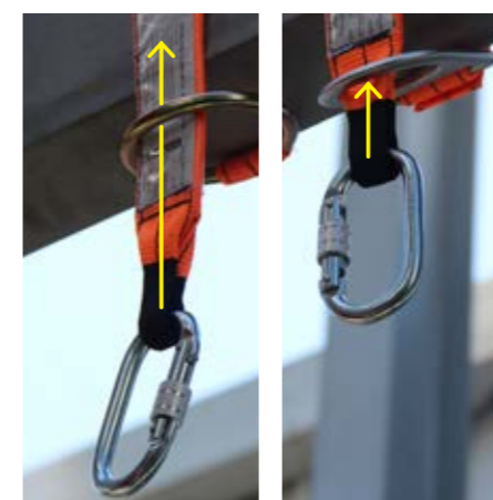
Carabiner can pass through large ring
